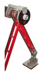
The control unit can read the two types of angular sensors, and can be used as heart of automatic test systems; it can be provided with analog output or with PWM motor control output.
